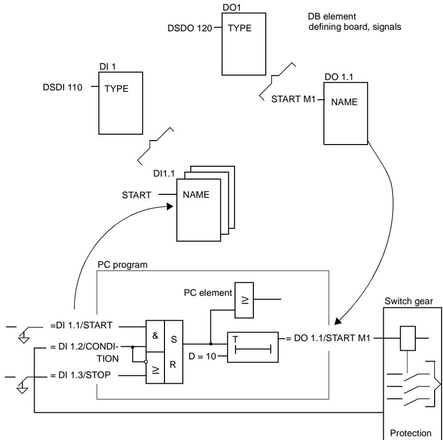
Figure 1-42. Simple Control Function Realized in AMPL
