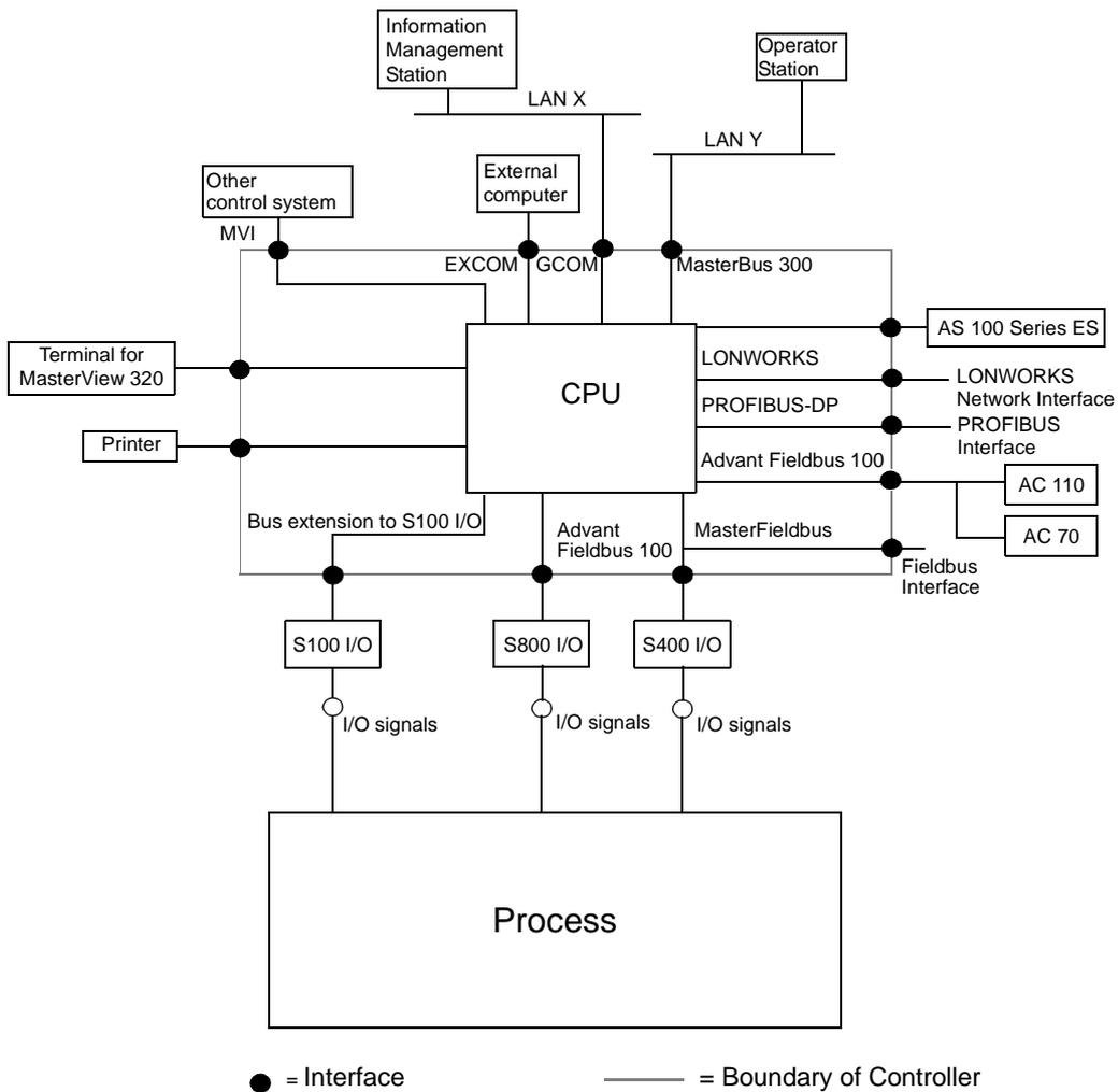
Figure 1-9. Advant Controller 450 Functional Interfaces
