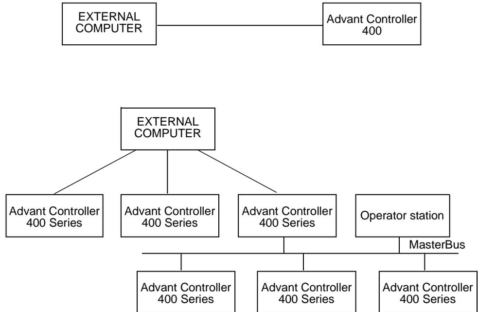
Figure 1-39. Alternative Connections of an External Computer to Advant Controllers
