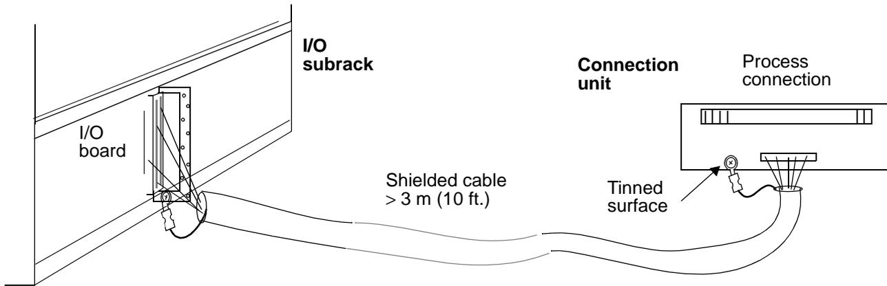
Figure 2-12. Grounding of Cable Shield, Connection Unit - I/O Board
