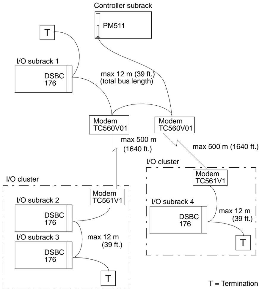
Figure 1-32. Example including Non-redundant Optical Bus Extension
