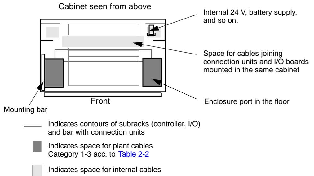
Figure 2-14. Assigned Space for Cables in a Cabinet
