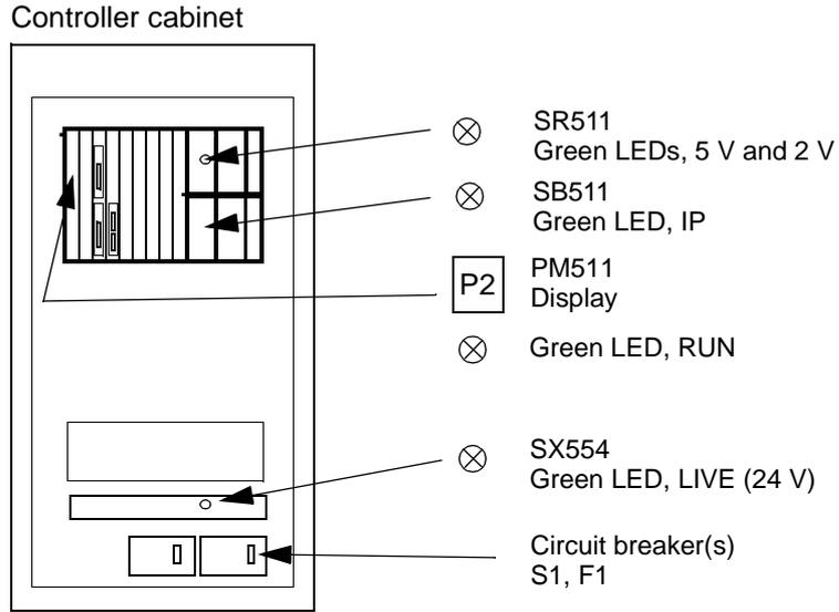
Figure 2-25. Power-up, Circuit Breakers and Positive Indications
