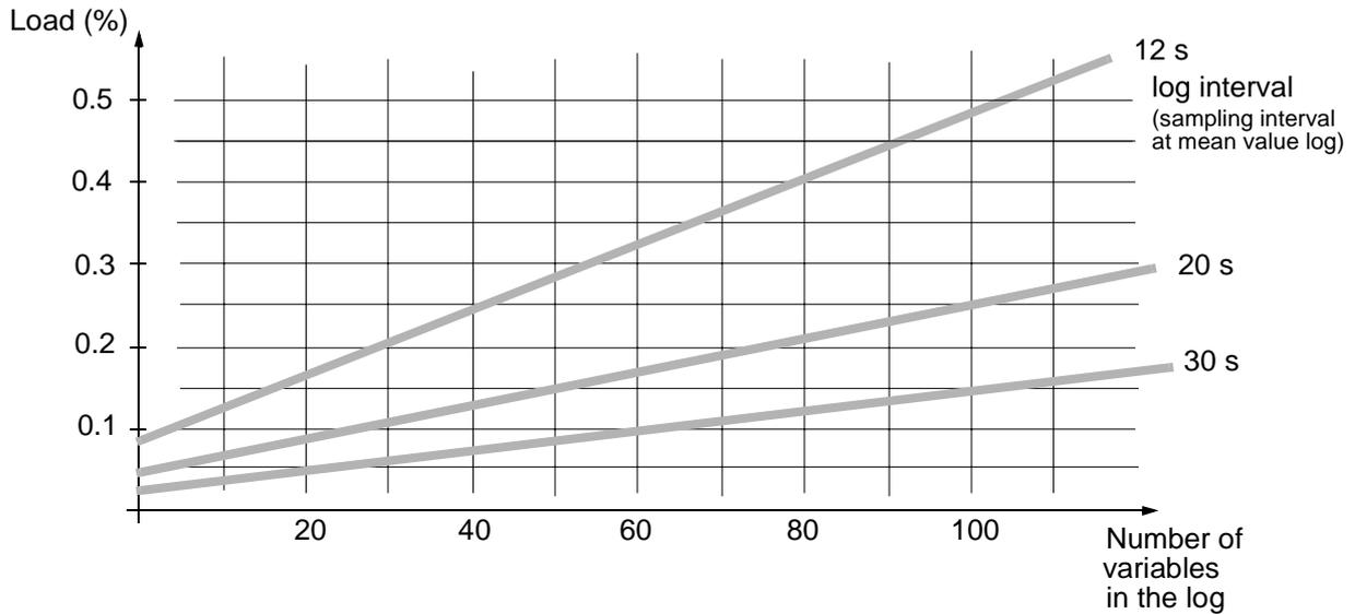
Figure 3-15. Load Caused by a Log (Medium Intervals)
