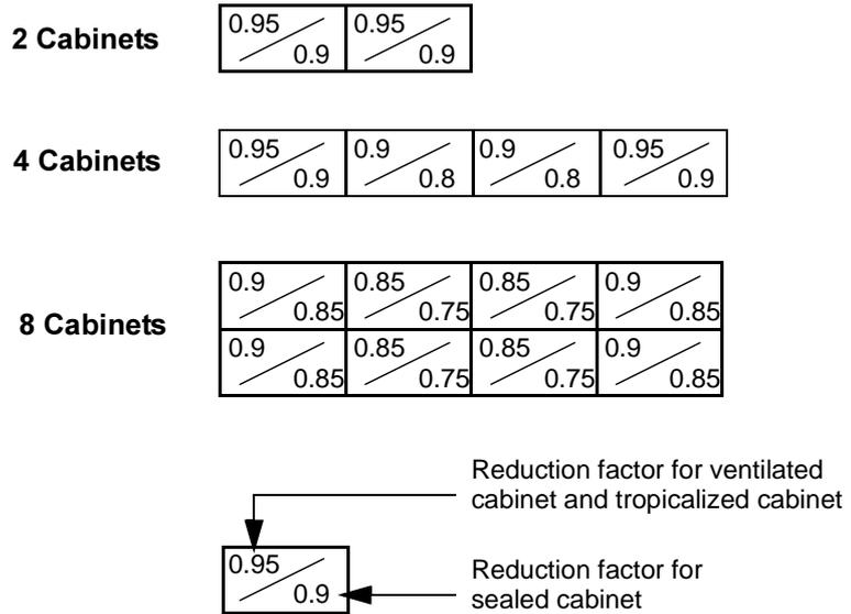
Figure 3-6. Reduction Factors for Cabinets Installed in Groups
