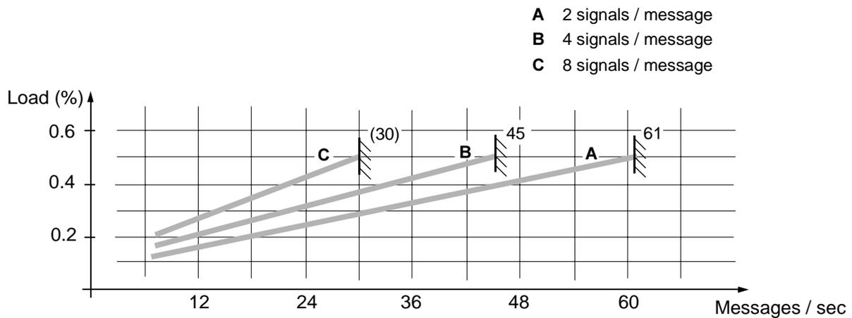
Figure 3-18. Load Caused by EXCOM, 1200 bit/sec.
