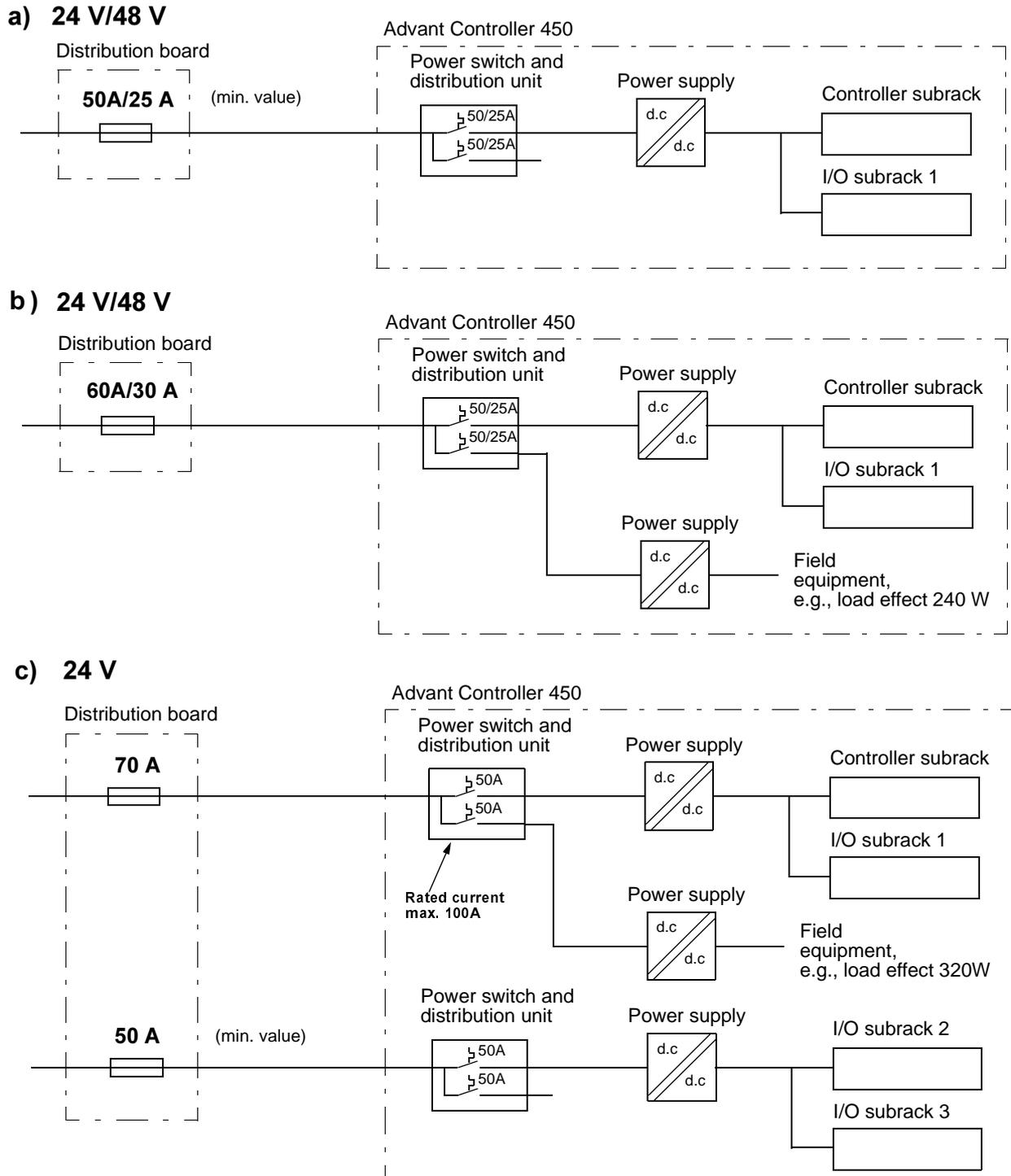
Figure 3-5. Examples of Distribution Board Fusing, d.c.
