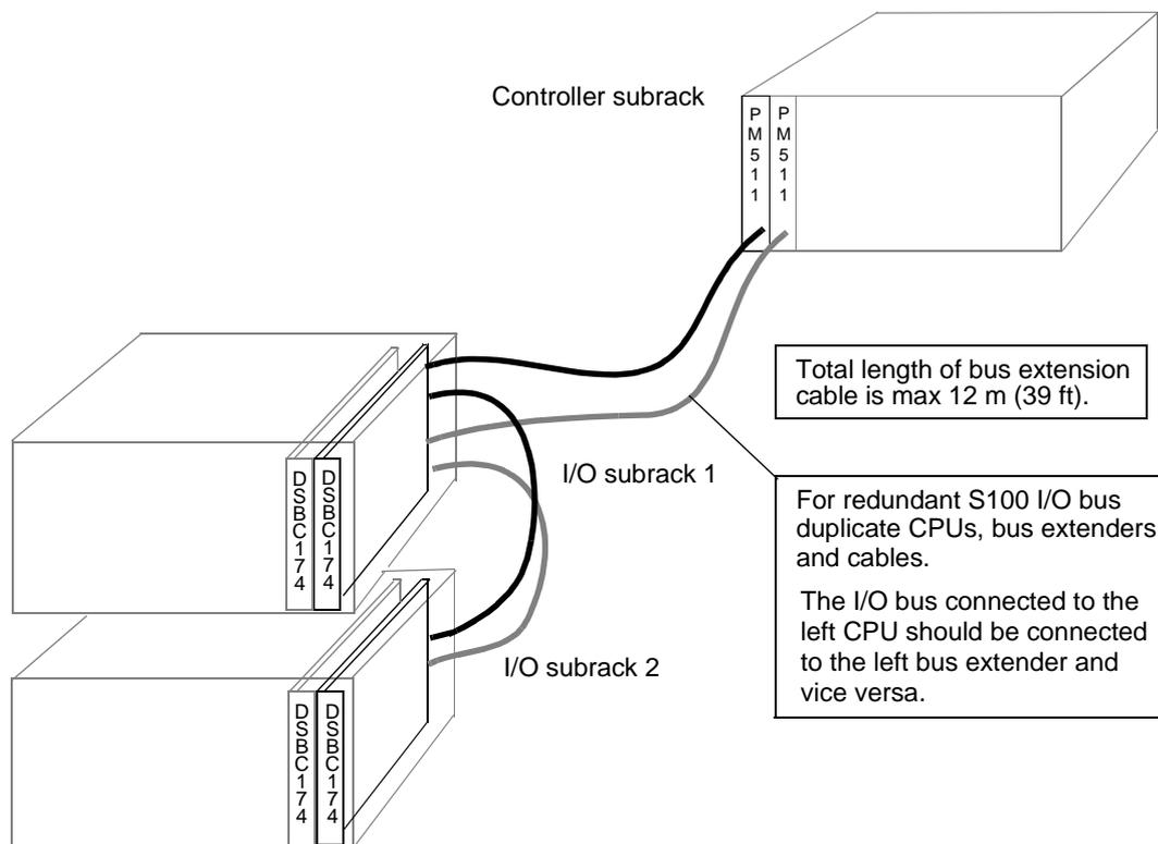
Figure 1-31. Example of Electrical Redundant Bus Extension
