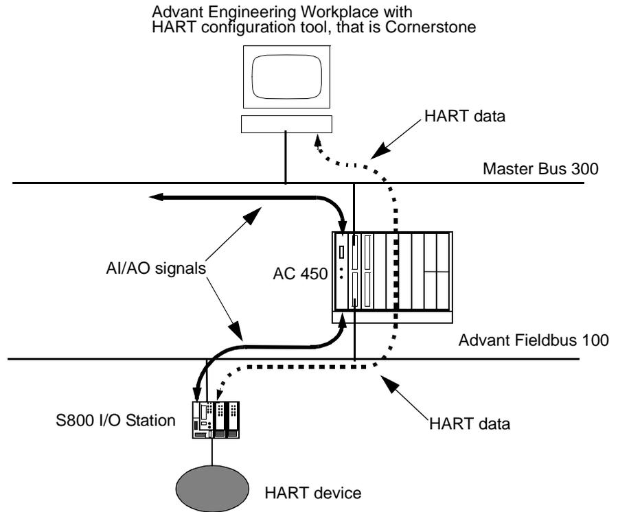
Figure 1-21. Principle of HART implementation using S800 I/O
