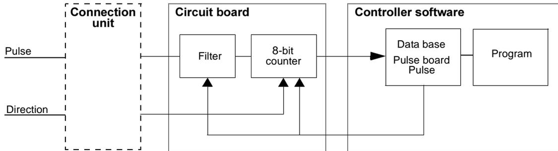
Figure 1-27. Pulse Counter Input Signal DSDP 110, Block Diagram
