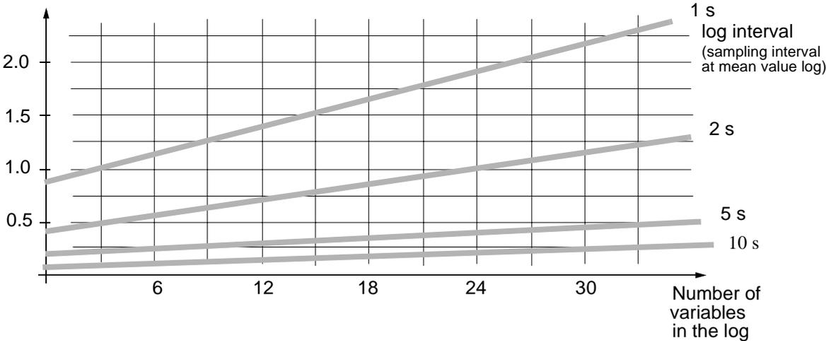
Figure 3-14. Load Caused by a Log (Short Intervals)
