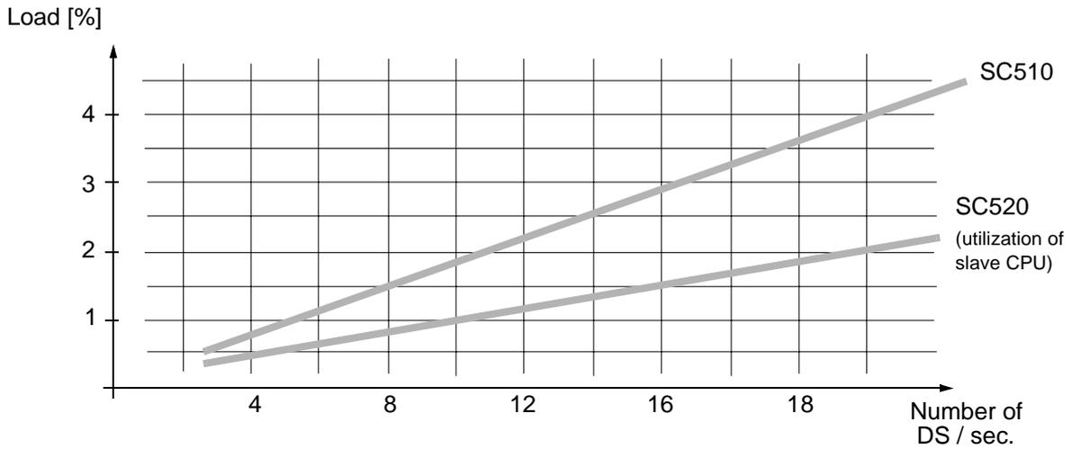
Figure 3-12. Load Caused by Receiving Data Set (MasterBus 300)
