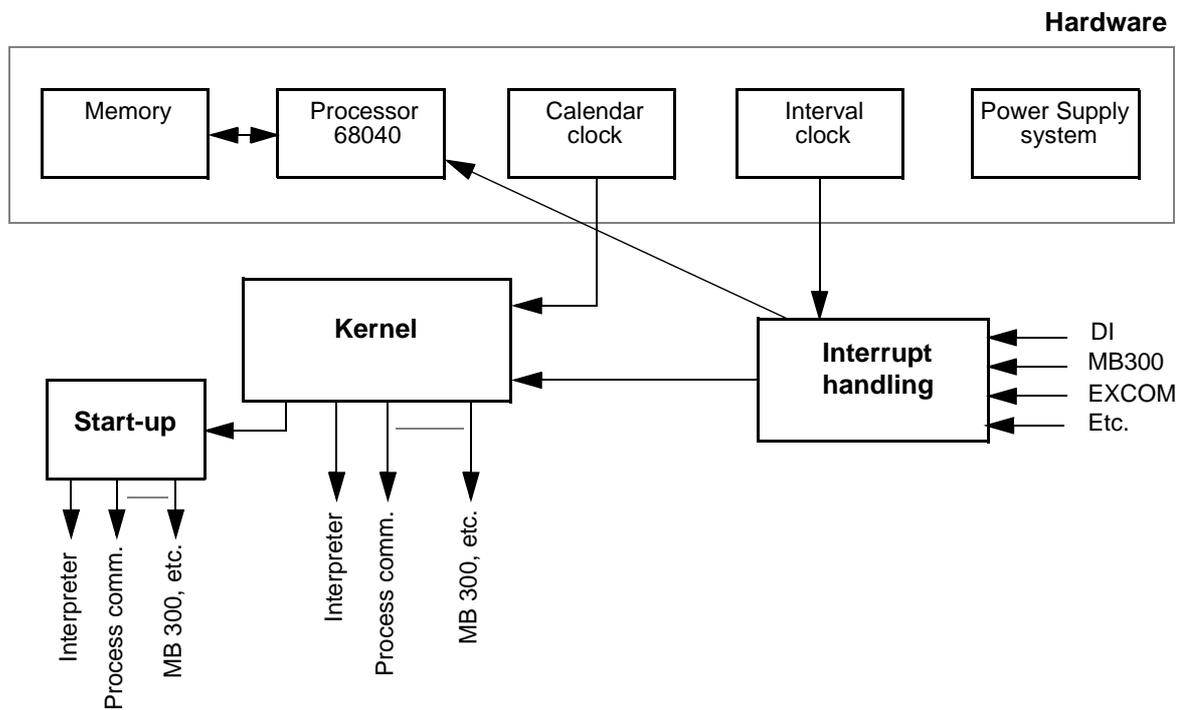
Figure 4-11. Survey of Processor Module and Operating System
