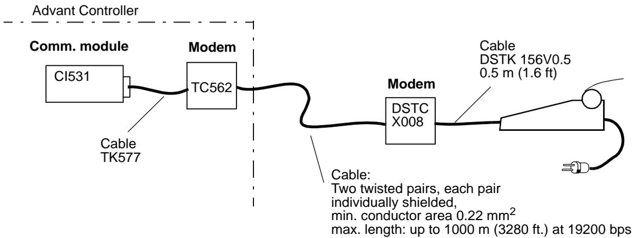
Figure 2-23. Long-distance Connection of Printer
