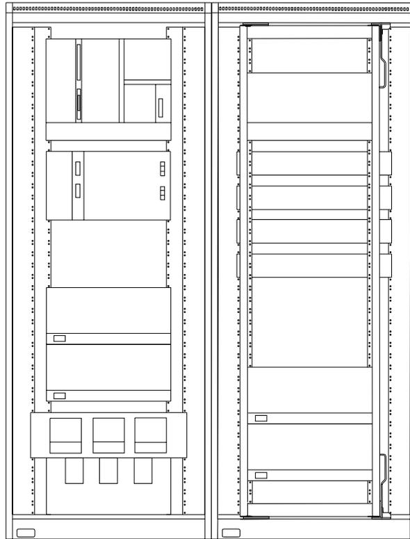
*Figure 1-4. Advant Controller 450 in RM500 Cabinet (doors opened) -
