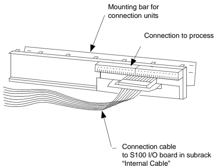
Figure 1-18. Example of Connection Unit for S100 I/O
