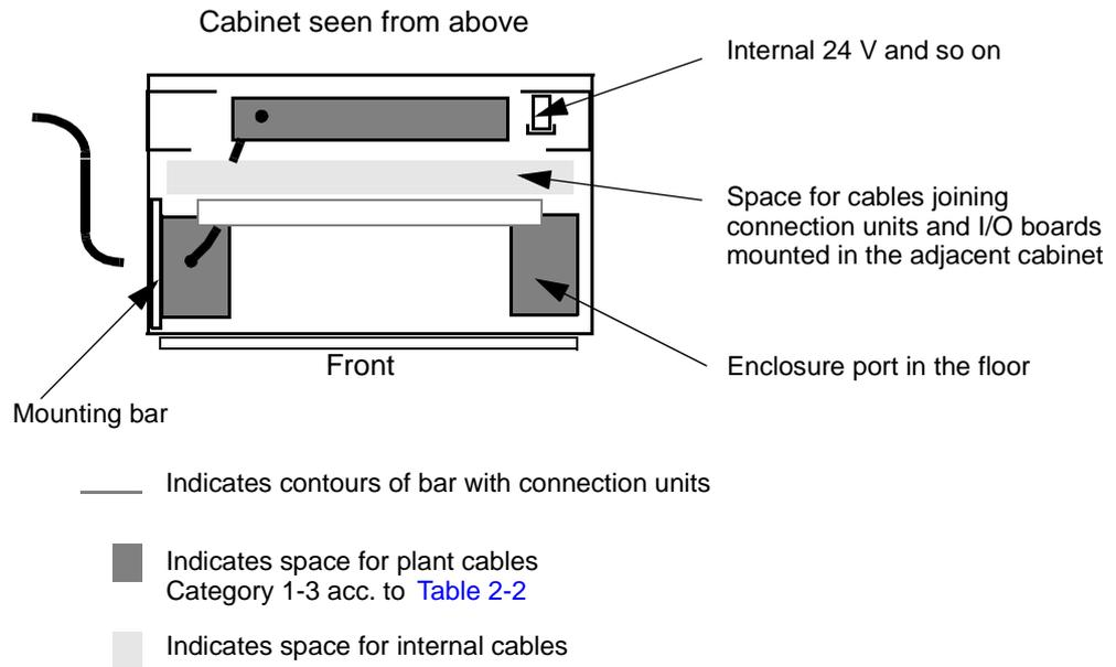
Figure 2-15. Plant Cable Routing in OOCU Cabinet
