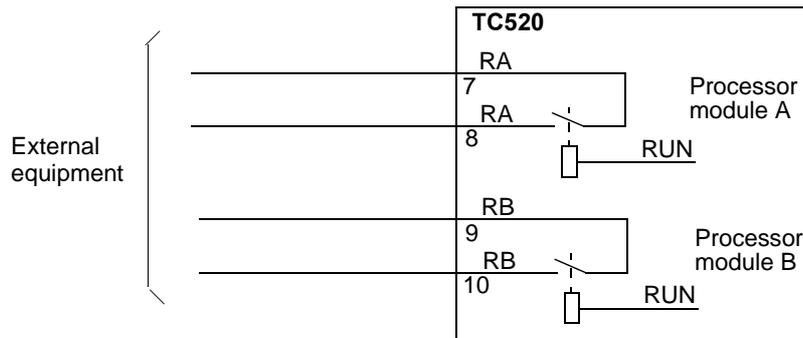
Figure 3-2. Run/Alarm Relay Connection
