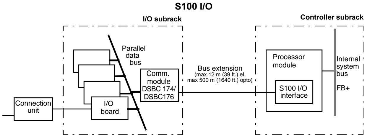
Figure 1-16. Input and Output Signal Paths (in principle)
