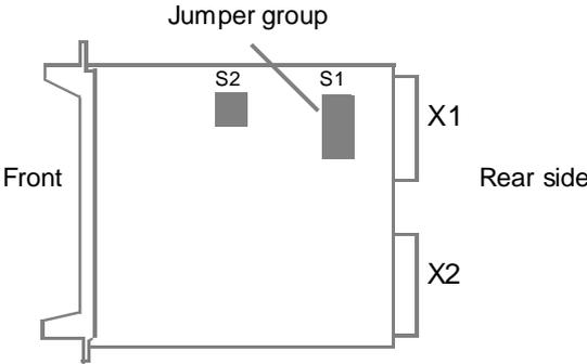
Figure D-11. Numbering of Connectors on the Rear Side
