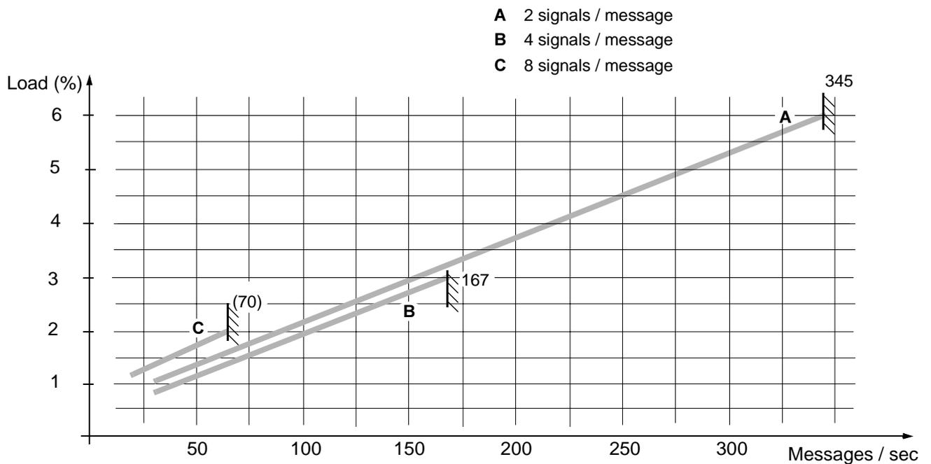
Figure 3-20. Load Caused by EXCOM, 19200 bit/sec.
