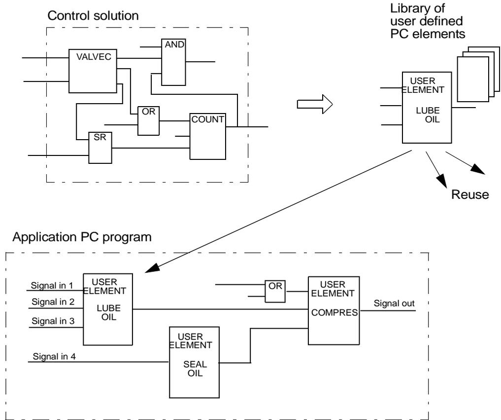
Figure 1-41. Process Objects Implemented as User Defined PC Elements
