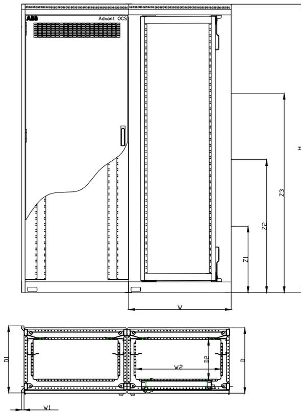
Figure B-2. Mounting Cabinets together - Screw Position
