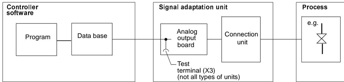
Figure 1-26. Analog Output Signal, Block Diagram
