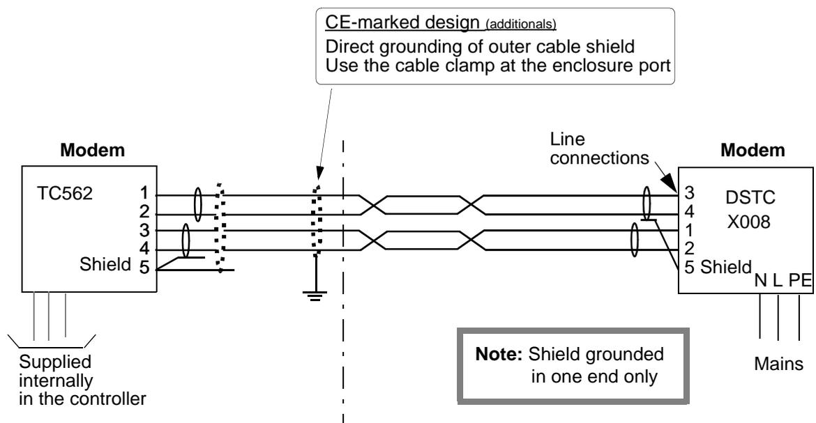
Figure 2-24. Connections and Grounding of Communication Cable Shields
