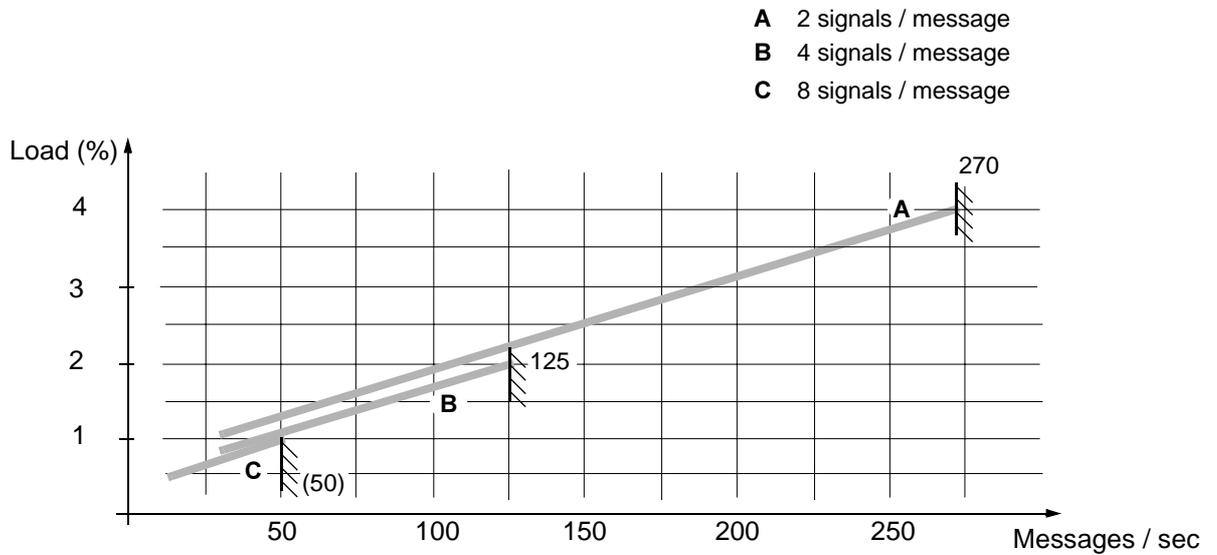
Figure 3-19. Load Caused by EXCOM, 9600 bit/sec.
