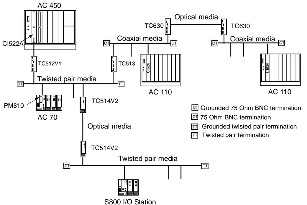
Figure 1-36. Media Conversion in Advant Fieldbus 100
