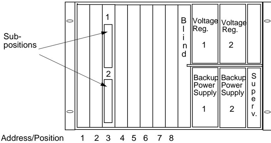
Figure D-5. Addresses in Controller Subrack 12 SU
