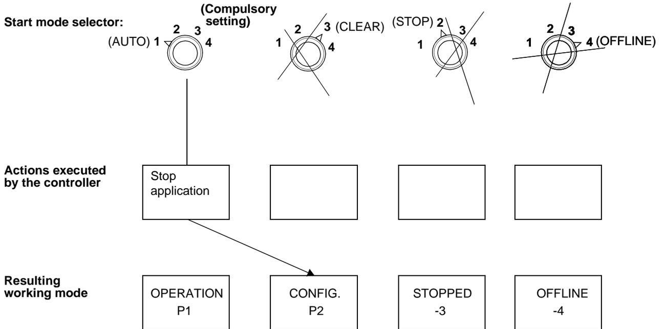
Figure 4-5. Working Mode Caused by ECONFIG
