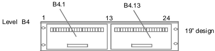
Figure D-13. Location of Connection Units on a Mounting Bar
