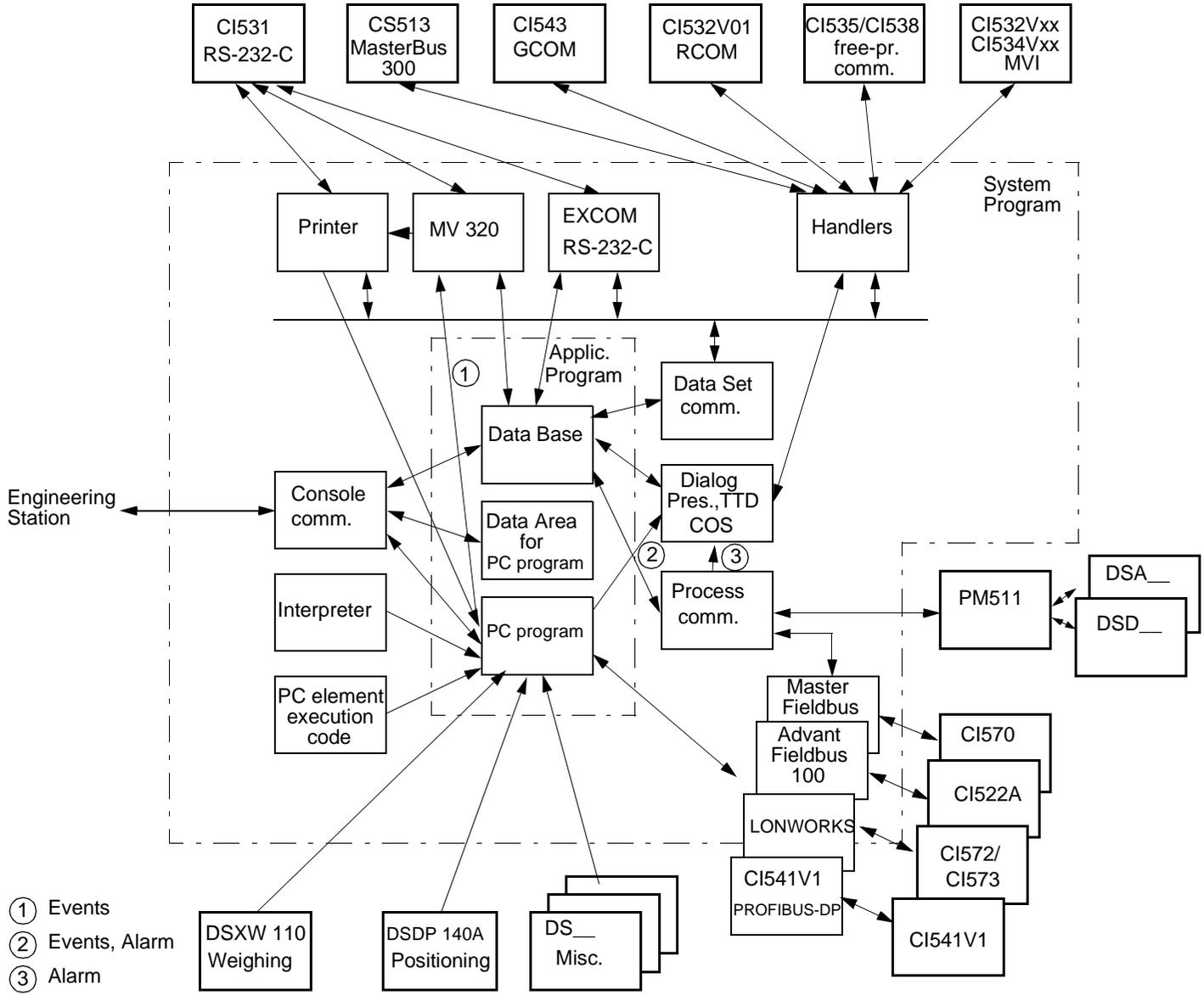
Figure 4-10. Advant Controller 450 - Survey of Software System
