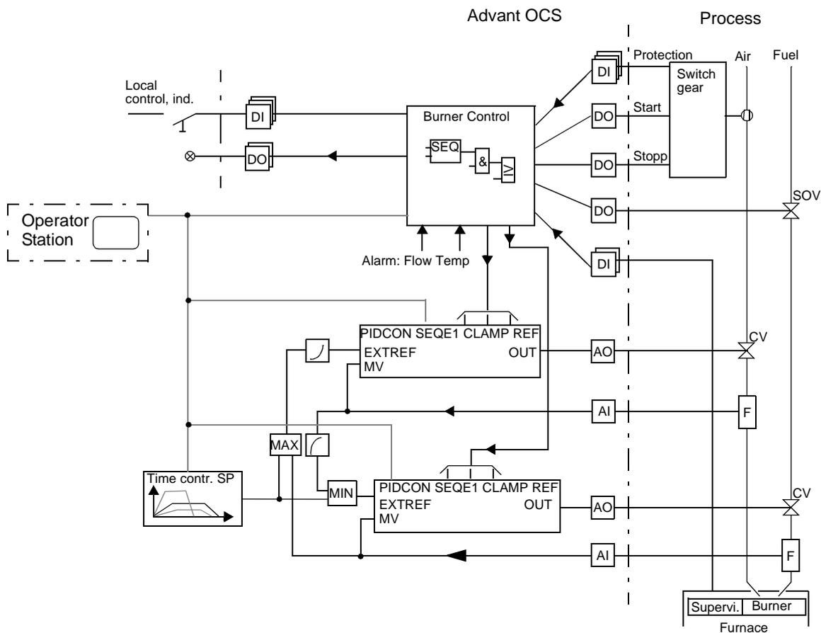
Figure 1-43. Principle of a Functional Unit Application
