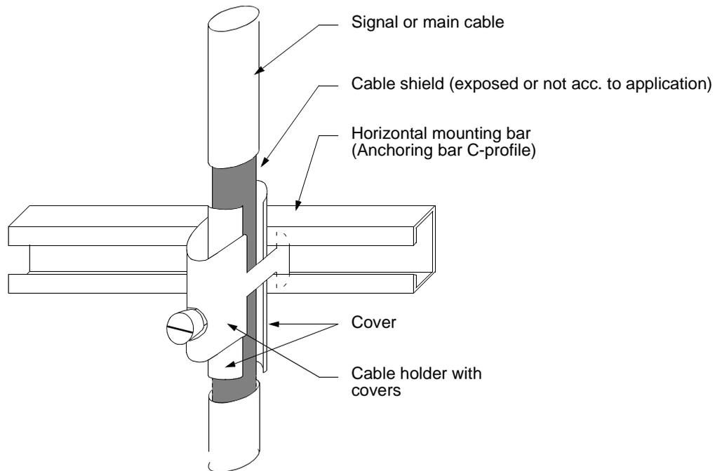
Figure 2-9. Handling of Cable Shields in a not CE-marked Cabinet
