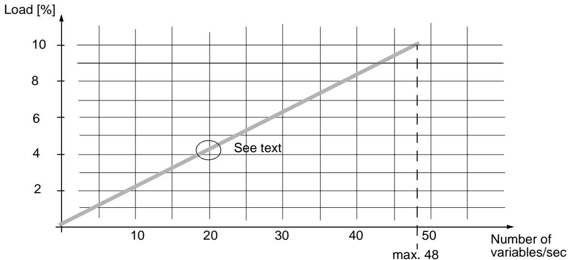
Figure 3-13. Load Caused by a MasterView 320
