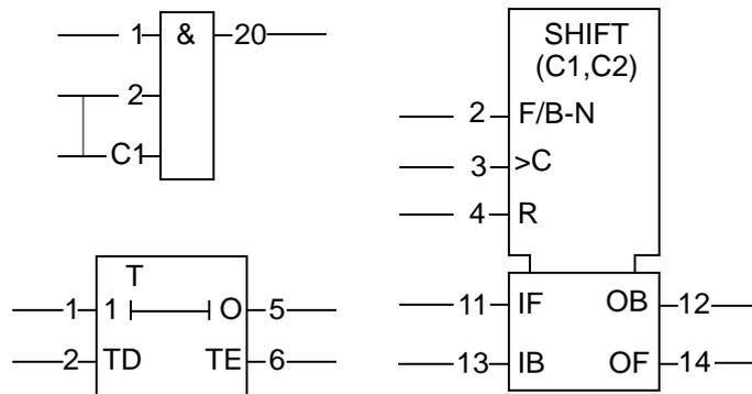
Figure 1-5. Example of PC Element (AND, TON, SHIFT)
