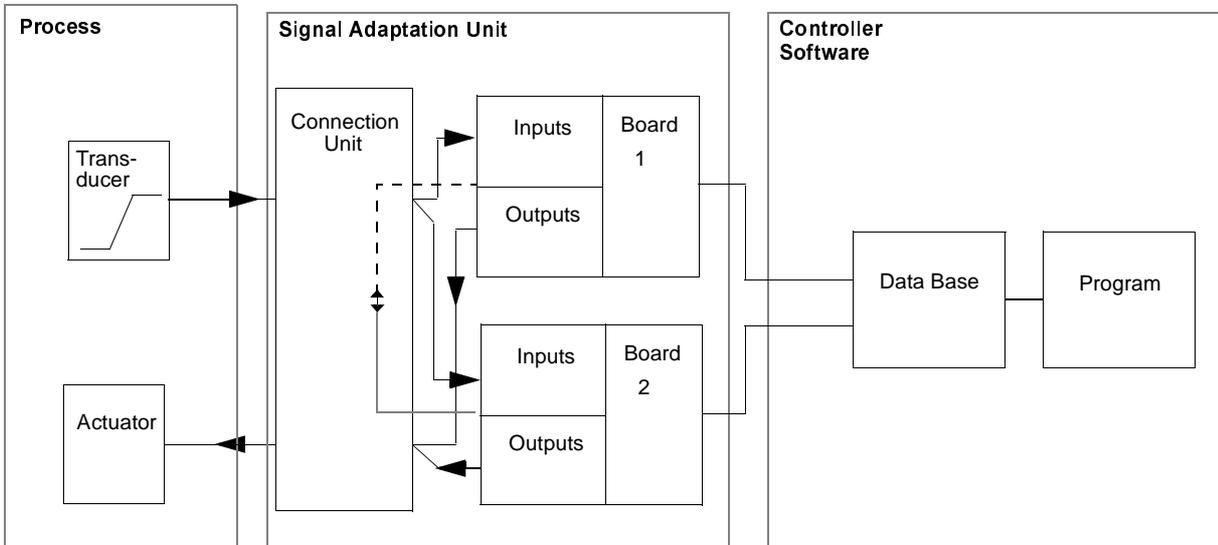
Figure 1-25. Analog Input/Output Signal with Redundancy, Block Diagram
