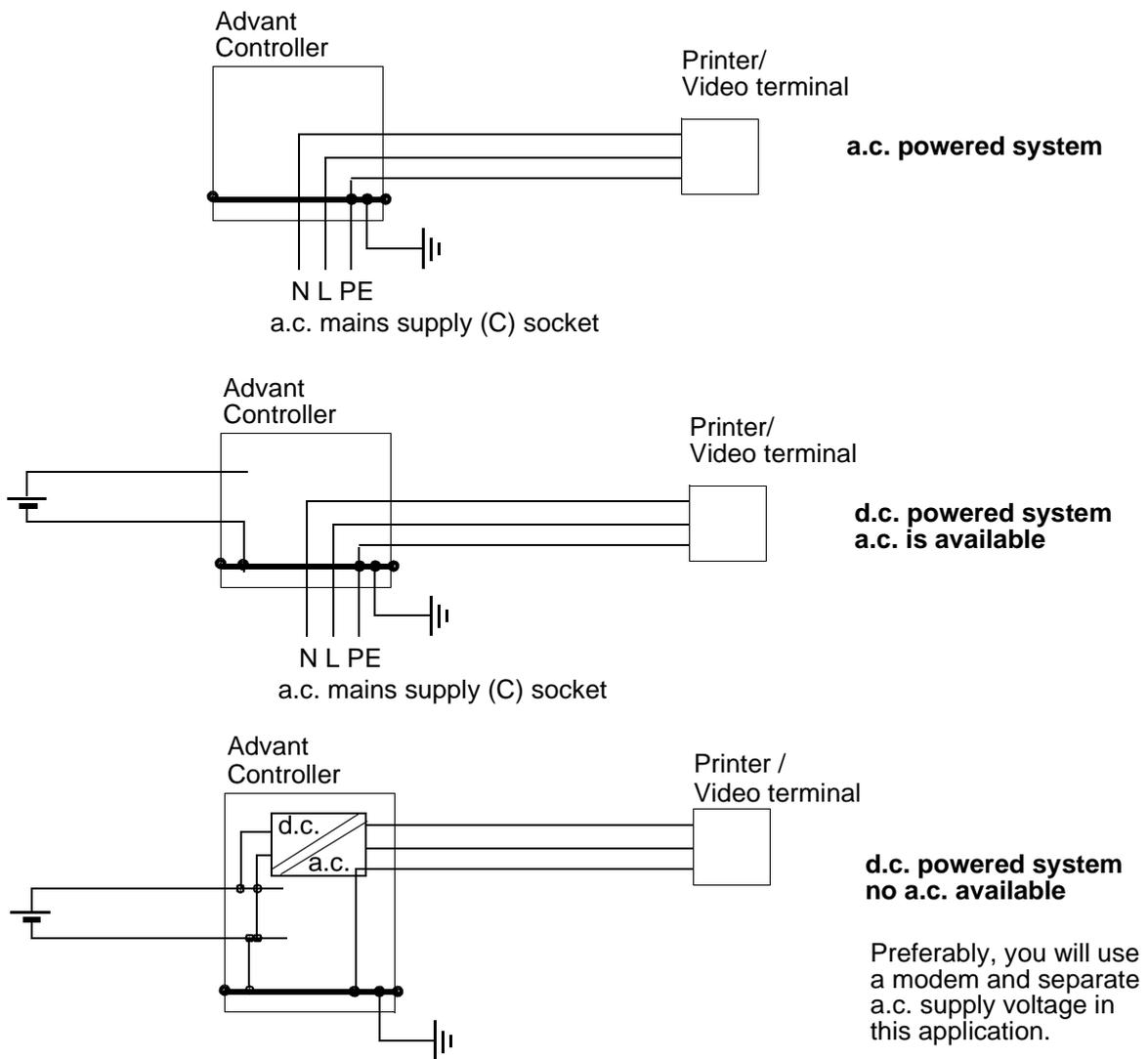
Figure 2-21. Supply of Peripheral Unit without Modem
