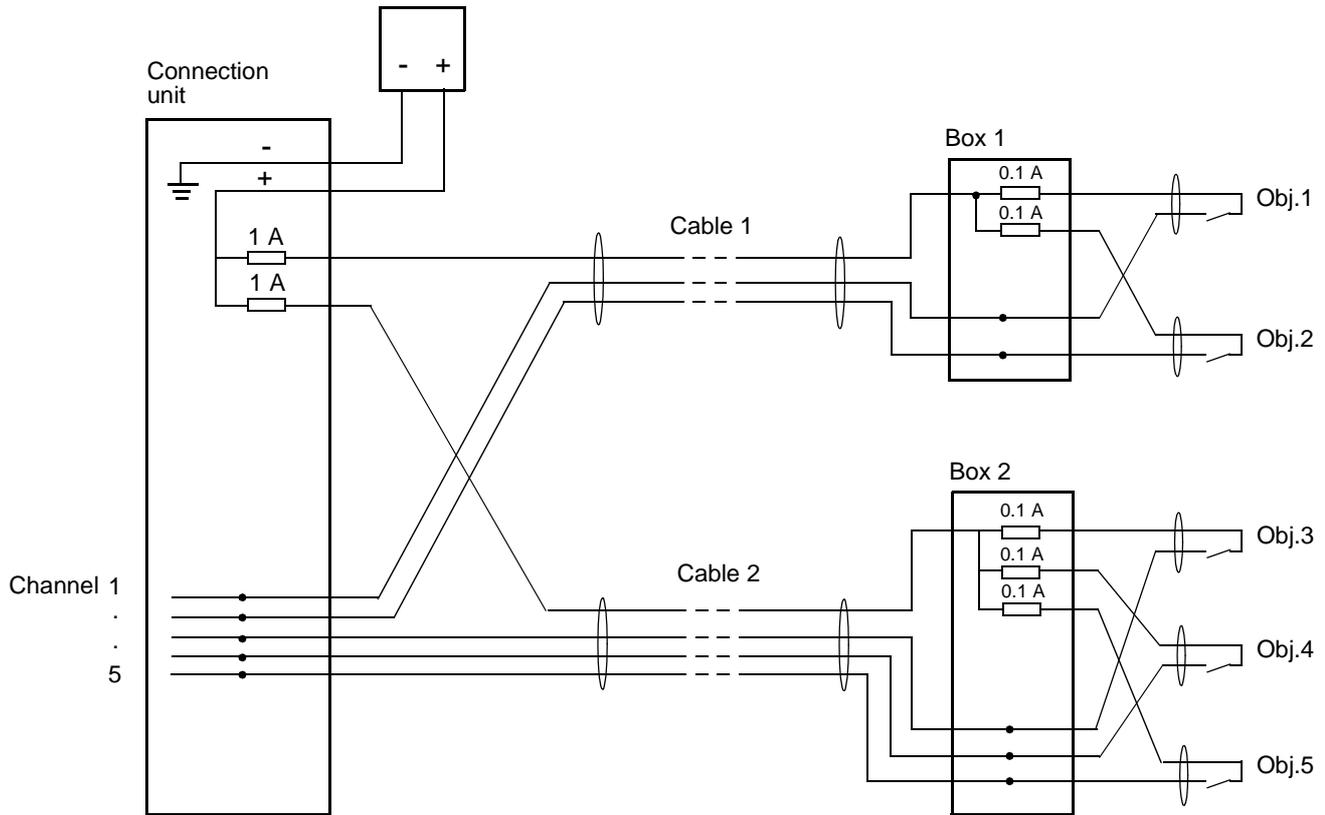
Figure 2-5. Connections with Multi-core Cable and Coupling Boxes
