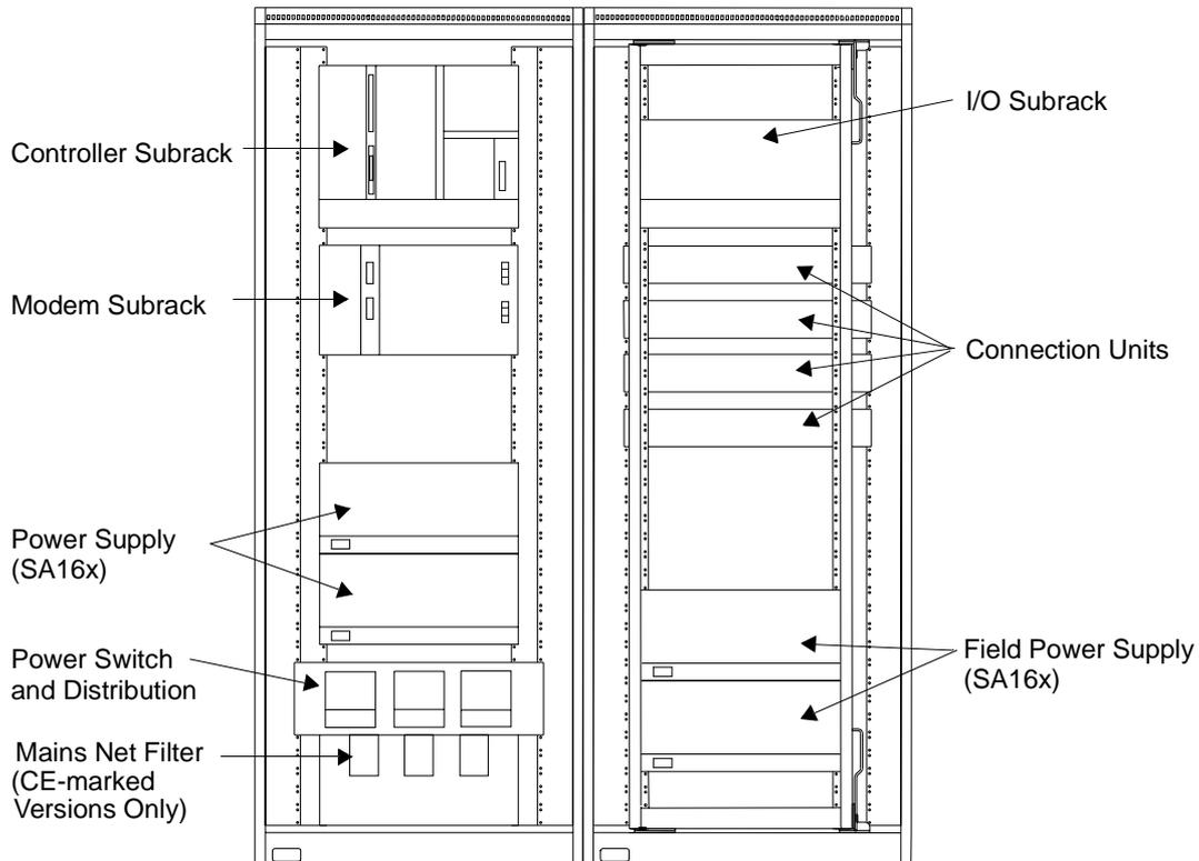
Figure 1-51. Typical Cabinet minimum Configuration, Redundant Power Supply
