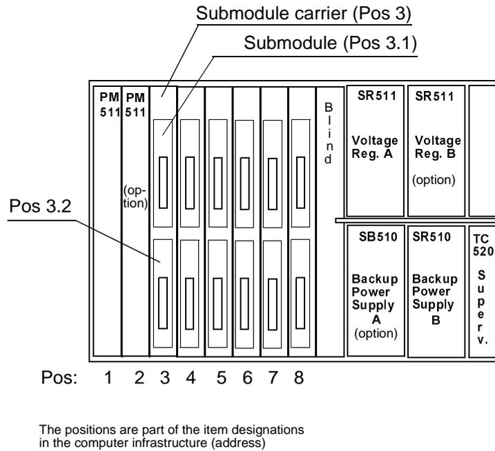
Figure 1-52. Advant Controller 450, Controller Subrack 9S
