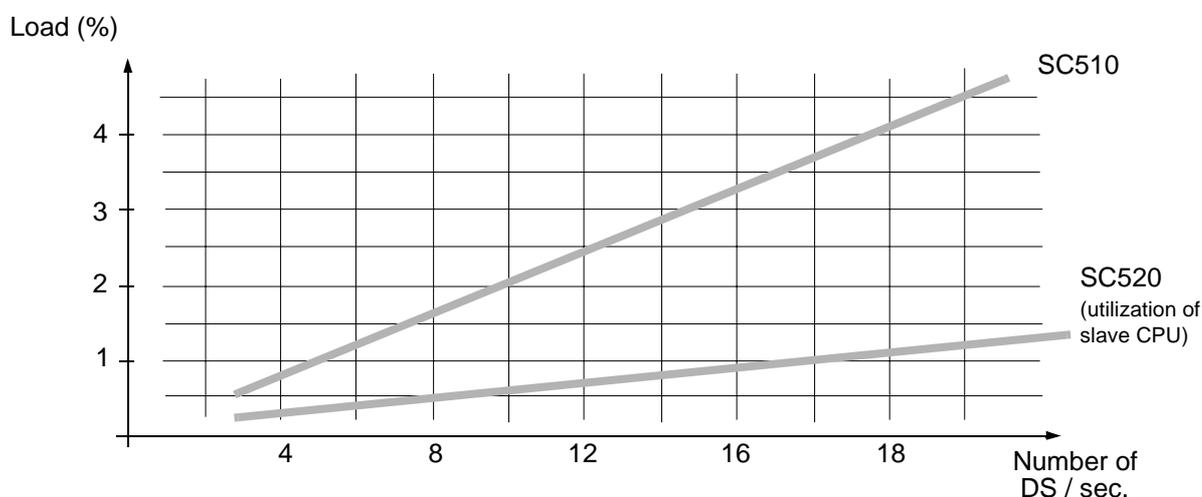
Figure 3-11. Load Caused by Sending Data Set (MasterBus 300)
