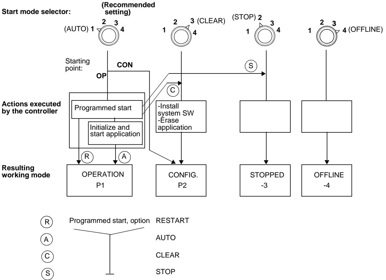
Figure 4-7. Programmed Start at Power-fail - Power-up
