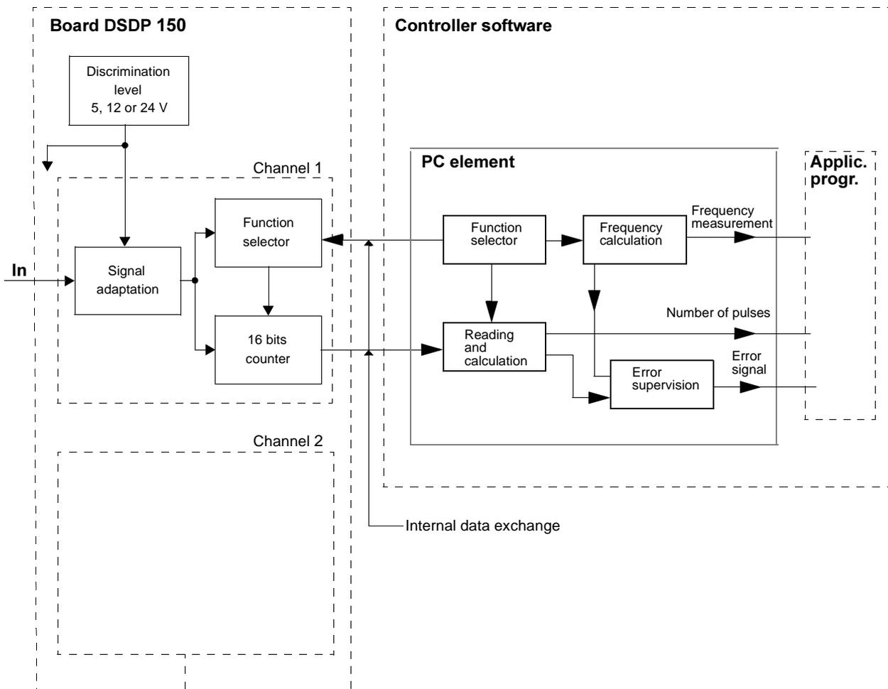
Figure 1-28. Pulse Counter Input Signal DSDP 150, Block Diagram
